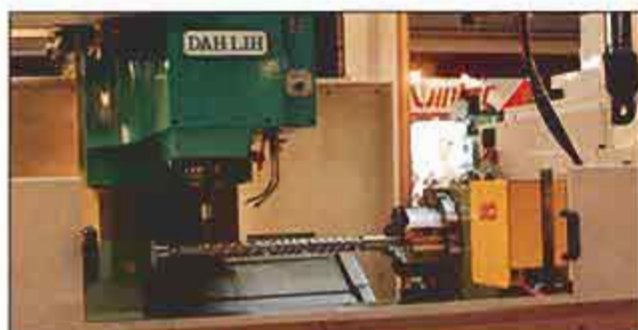
CNC-321R + TSA-826 (Tallstock) Application: Vertical Machining Center
