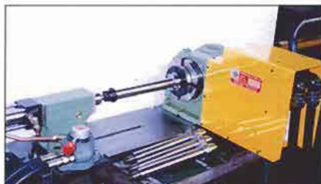
CNC-151R + PTSA-530 (Power Tallstock Hydraulic) Application: Vertical Machining Center
