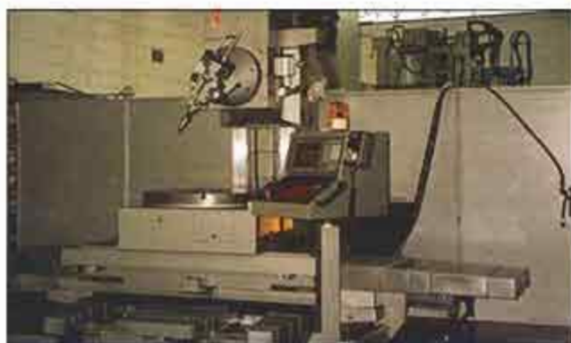
CNC-631RV + CNC-401RV Application: Horizontal Machining center or conventional machine
